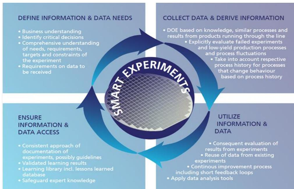
The smart experiments concept: A broad-based holistic approach considering the whole lifecycle of data and information in the fab (© Fraunhofer IISB)
