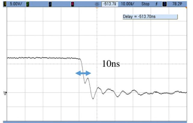
Fig. 8  $V_{DS}$  fall time  $V_{in} = 12V$
