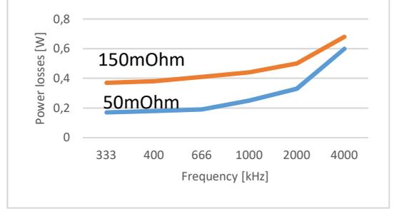
**Fig. 4 Power losses on power switch vs frequency**
