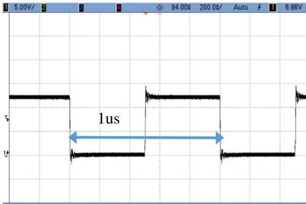
Fig. 11  $V_{DS}$  on power switch
