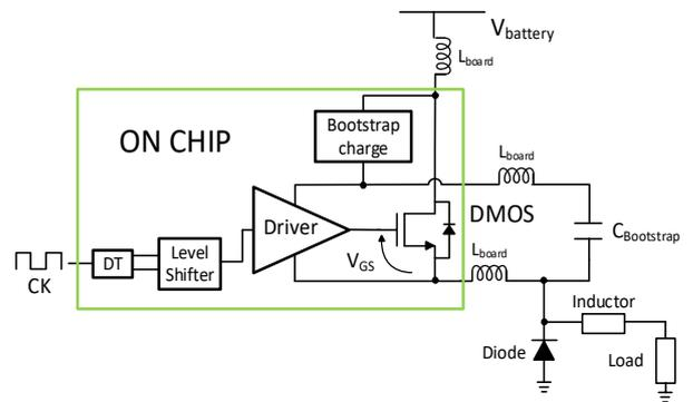
**Fig. 1 Block diagram of gate driver**
