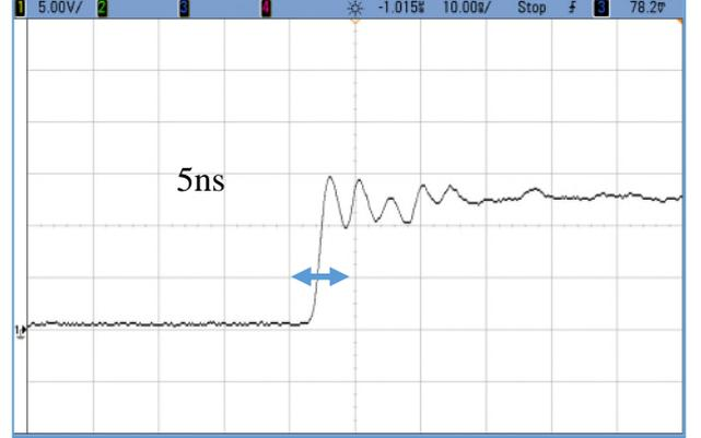
Fig. 7 VDS rise time  $V_{in} = 12V$
